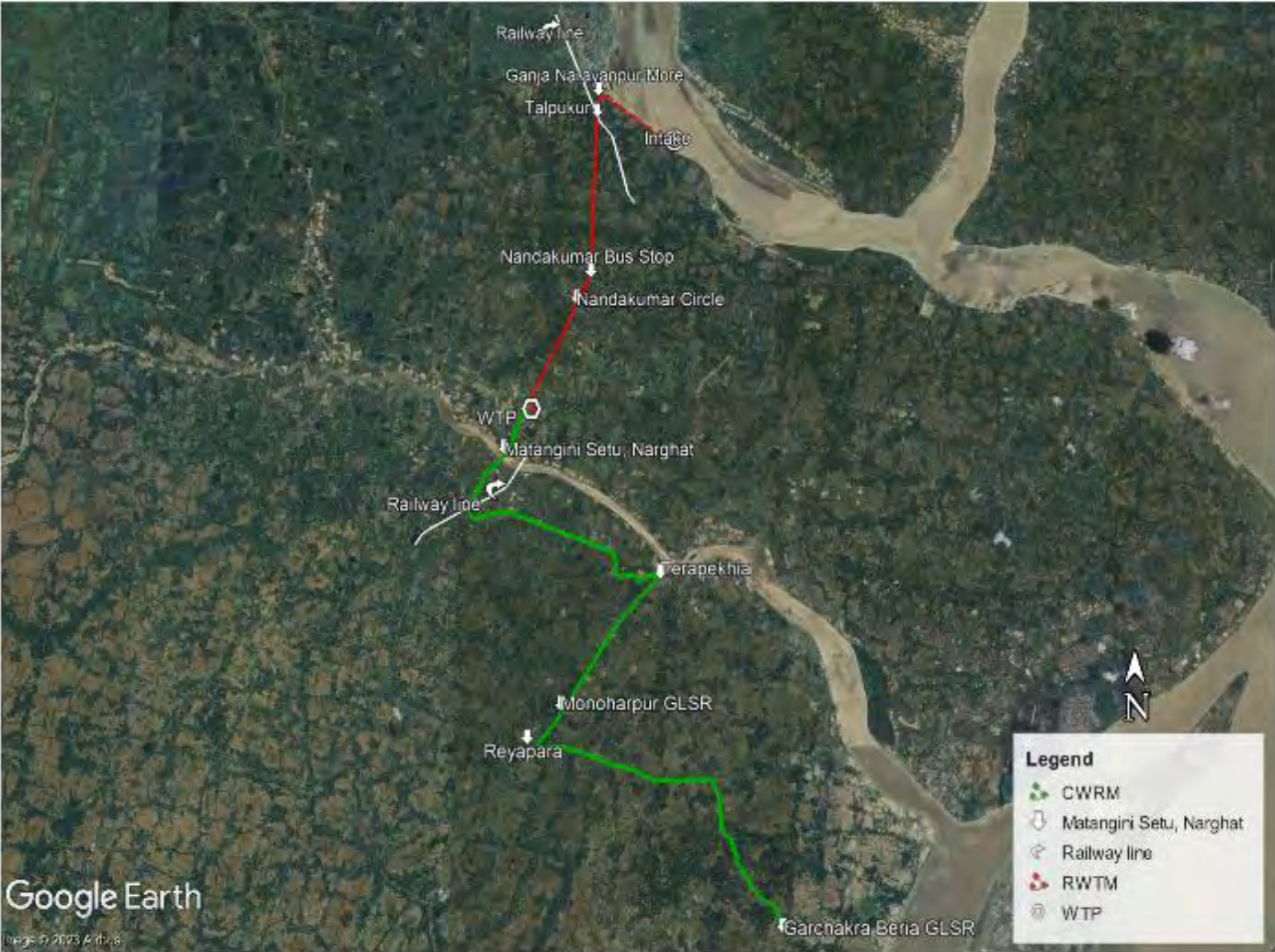
Figure 3.2: Google map showing raw water transmission pipeline from intake to WTP and also clear water main to both GLSR with marking of location.
